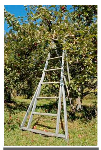
Orchard ladders should only be used for tree harvesting and pruning tasks. They should be set on soft ground.
