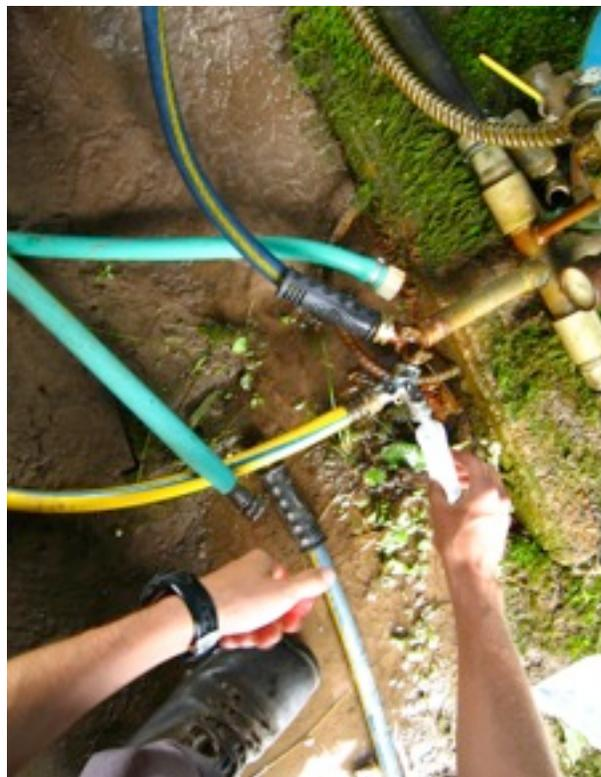
Let the water run for 3 minutes before taking a sample to ensure you are testing the water from the well.
