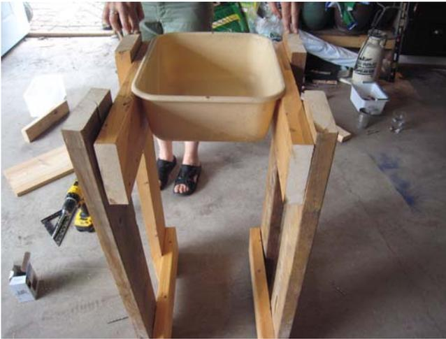
**4. Figure out how wide to cut the width-wise crosspieces.** Placing our dishpan on the “drawer slides” we measured and determined that crosspieces of 14.5” would work. We cut 4- 14” pieces of wood. This time we used 2x4s.
