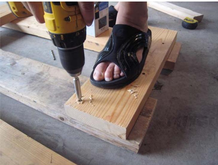
Here you can better see how we placed the top cross piece down from the top to be the dishpan drawer slide.
