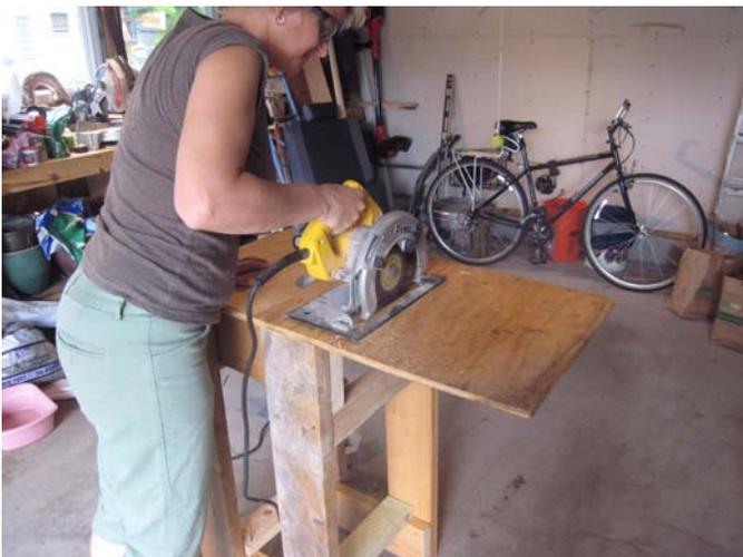
**7. Next, cut a scrap of plywood, old countertop, or some other flat material (not glass) to fit the top of the stand.**
